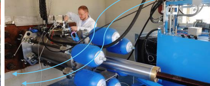
Hopkinson Bar facility (HOPLAB)
